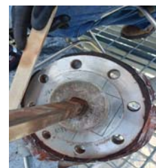
Check and clean probe pressure unit 1
