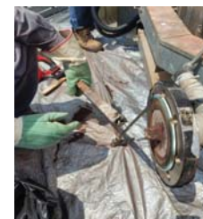
Check and clean probe pressure unit 2
